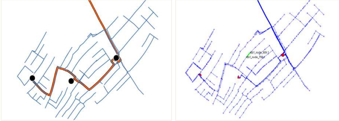
Figure 22. Feeder 1 GIS layout without secondary nodes (left) and its OpenDSS models with added secondary nodes (right)
