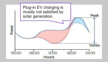
**Smart charging** allows plug-in electric vehicles to consume more electricity when renewable generation is high. Additional case for dynamic charging when rates are set for the time of the day (i.e. no variation on day-to-day basis)
