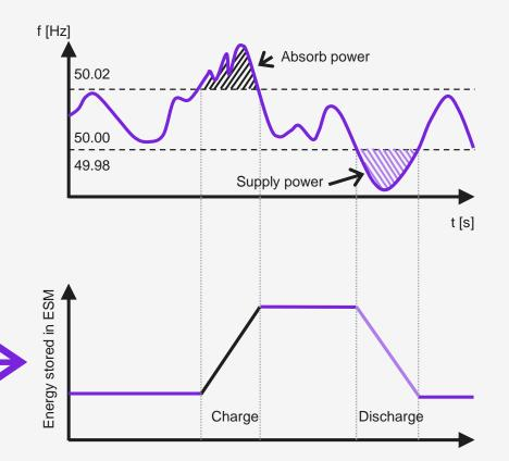
The electricity storage system is charged or discharged in response to an increase or decrease, respectively, of grid frequency. This approach to frequency regulation is a particularly attractive option due to its rapid response time and emission-free operation.
